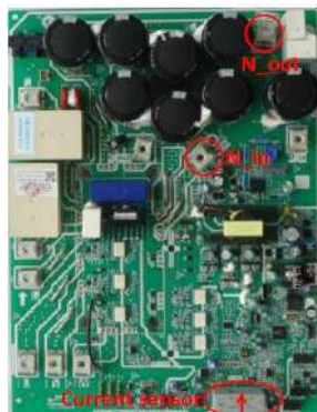
Figure 6-2.5: DC detection wire connection method
