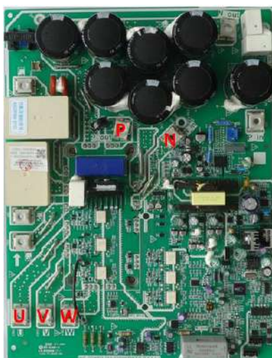
Figure 6-2.1: Inverter module terminals
