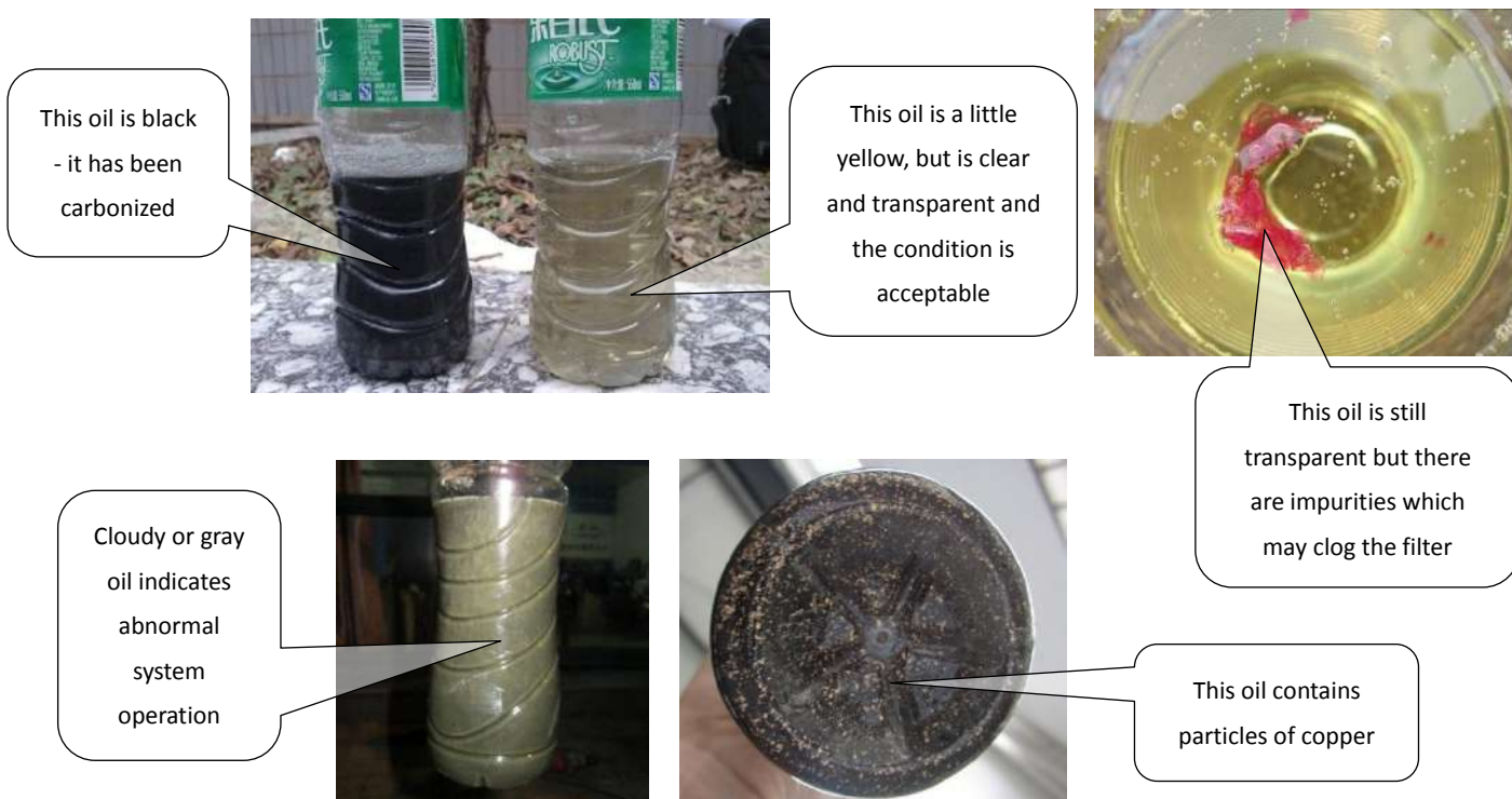
Figure 6-2.10: Inspecting compressor oil
