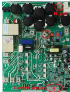
Figure 6-2.2: DC detection wire connection method
