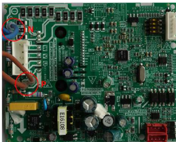
Figure 6-2.12: Fan module P N terminals
