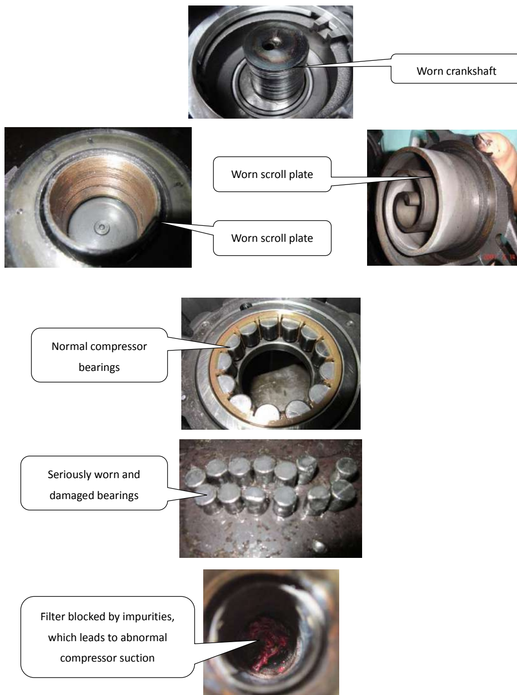
Figure 6-2.11: Effects of spoiled compressor oil
