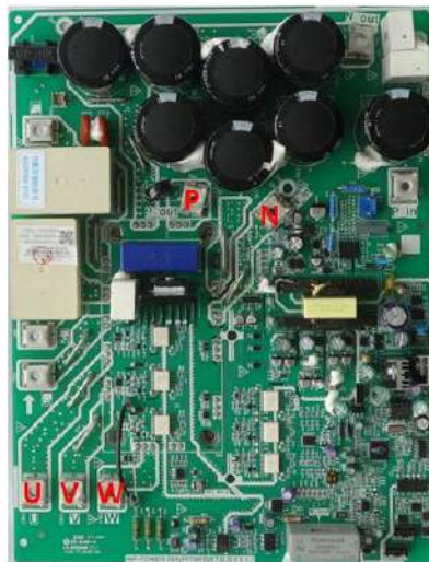
Figure 6-2.6: Inverter module terminals
