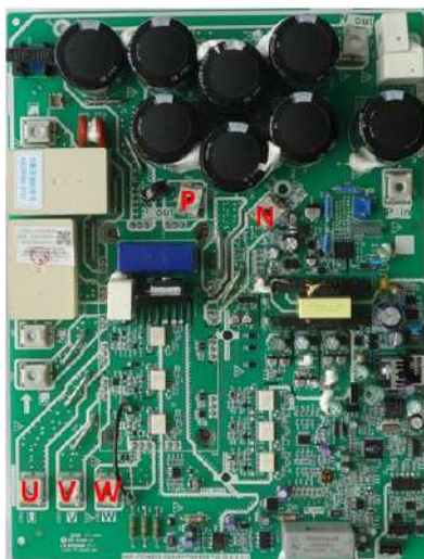
Figure 6-2.7: Inverter module terminals
