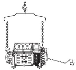
**NOTE:** The spreader bar in Figure 12 is a representation only and may not reflect the appearance of the actual spreader bar needed.
