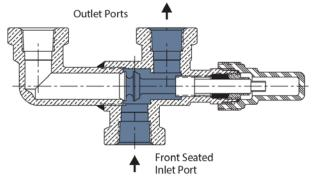
Figure 18: Three-Way Valve, Back Seated Position
