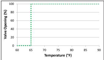
As shown in Figure 38, the default temperature at which the valve opens completely is 65°F. This temperature is the Valve SP (also called Valve Target) and is adjustable.
