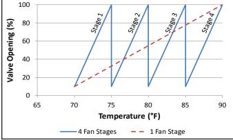
As shown in Figure 41, the default minimum and maximum valve opening positions are 10% and 100%, respectively. These minimum and maximum positions are adjustable anywhere between 0% and 100%. Additional fans stage on when the valve opening position reaches the maximum value that was set.
