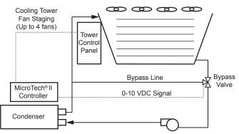
Figure 41: (III) VALVE STAGE -
