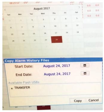
The Alarm History Screen can be used to download the trend history (Figure 55) or the alarm history (Figure 56) via USB. In order to download the trend or alarm history, first insert a USB drive into the left side of the monitor as seen in the following figure.
