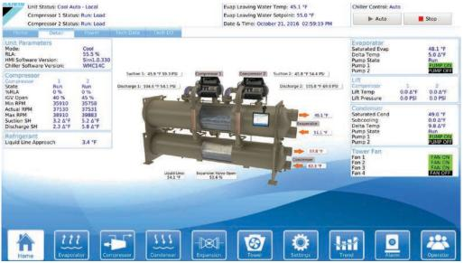
Data for all compressors is shown simultaneously on the Detail View Screen. If the unit is a dual compressor unit, pressing the COMP button in the lower-left hand corner of the screen will generate additional statuses.
