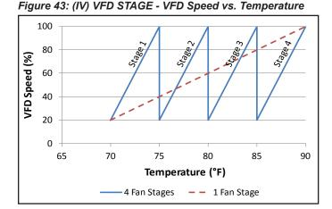
As shown in Figure 43, the default minimum and maximum VFD speeds are 20% and 100%, respectively. These minimum and maximum values are adjustable anywhere between 0% and 100%. Additional fans stage on when the VFD speed reaches the maximum value that was set.
