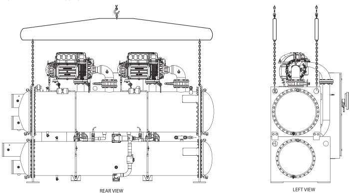
**NOTE:** The spreader bars in Figure 5 are a representation only and may not reflect the appearance of the actual spreader bars needed.
