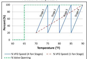
As shown in Figure 45, the default minimum and maximum VFD speeds are 20% and 100%, respectively. These minimum and maximum values are adjustable anywhere between 0% and 100%. Additional fans stage on when the VFD speed reaches the maximum value that was set. In addition, Figure 45 shows that the default temperature at which the valve opens completely is 65°F. This temperature is the Valve SP (also called Valve Target) and is adjustable. **BAS Alternate**
