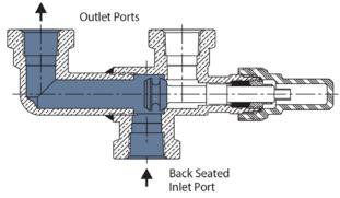
When the valve stem is not pushed forward or pulled back completely, the valve is in "Mid Position," as shown in Figure 19.
