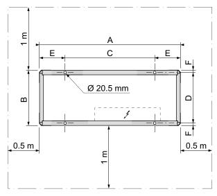
Free space to be maintained to allow sufficient room for maintenance of the unit.
