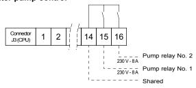
Connect the supply to the pump relays between the terminals of the connector on the main board.
