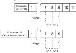
Connect 1 to 4 contacts to the terminals of the connector of the CPU board according to the number of the compressors to be shed. 1 contact per compressor (contact free of any polarity and of good quality).
